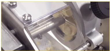
The general consistency of the extruded dough is much drier than the dough used with a sheeting machine. The mixture is forced through bronze dies that can create hundreds of different pasta shapes!
